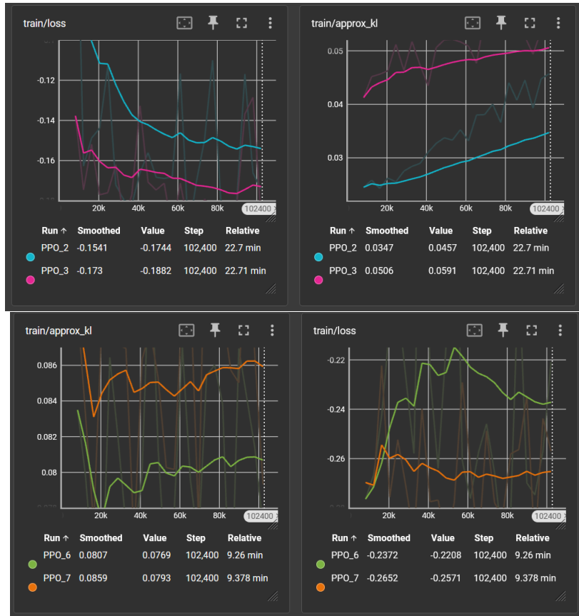
Figure 1: Loss and KL-divergence results of agents trained with a discrete action space (top) and a continuous action space (bottom) for about 400,000 time steps. Each graph plots the metrics of the last 200,000 time steps for the agents.
